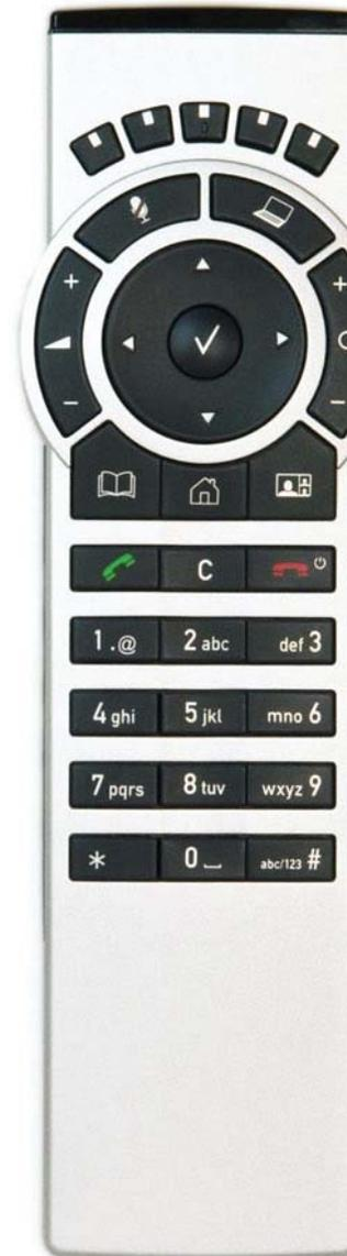
The function keys in the upper part of the remote control reflect the softkeys on screen
